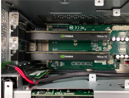
3. Use a cross-head screwdriver to tighten the screws to secure the graphic card holder.
