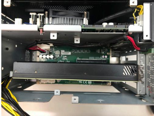
3. Use a cross head screwdriver to tighten the screws to secure the graphic card.
