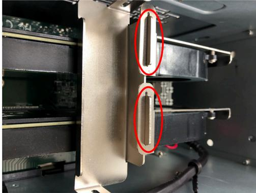
5. Use a cross-head screwdriver to tighten screws on the graphic card bracket.
