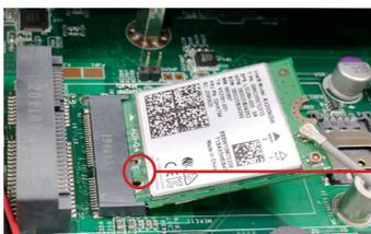
The module's key notch should meet the connector's break.
