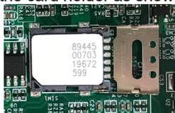
5. Close the SIM card holder door and slide the door to the LOCK edge to lock into place.
