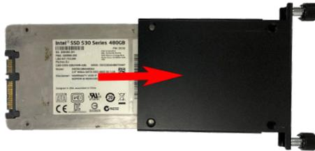
3. Fix the storage device in place by fastening the four screws of the bracket.
