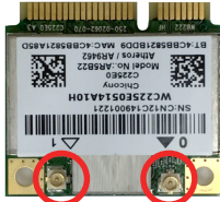
U.FL connector labeled "1" for main W-Fi antenna
